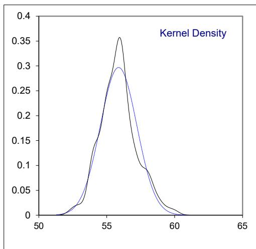
Determination of Kinematic Viscosity at 40°C on sample #22005; result in mm<sup>2</sup>/s
